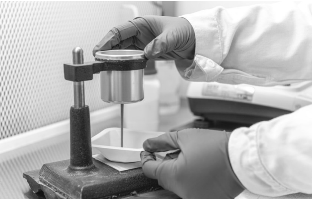
Testing the flowability of metal powder materials
