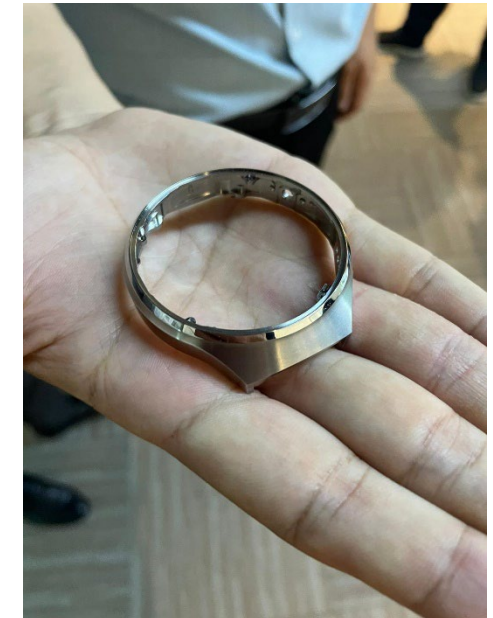
Mobile phone and smart watch frames produced with Tekna Titanium powder Photo courtesy of a Tekna customer in Asia
