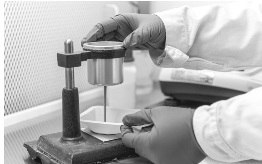
Testing the flowability of metal powder materials
